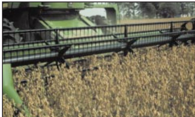
Figure 14.2. Reel adjustment for gentle soybean handling is more critical after soybeans have dried down once (or with certain Maturity Group IV varieties).
